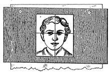
making a cross. Two small holes are drilled in the plate, one on either side of the aperture. The slip of brass is laid on the portrait with the aperture over its face. It is turned about until one of the cross threads cuts the pupils of both the eyes, and it is further adjusted until the other thread divides the interval between the pupils in two equal parts. Then it is held firmly, and a prick is made through each of the holes.
